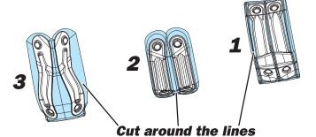
Installation of body stiffeners for BORA 1/8 onroad bodyshell
